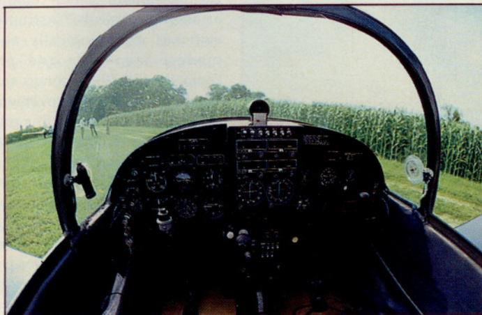
Larger pilots may find the Falco cockpit cramped, but the visibility is excellent. Scott has replaced his original instruments with more modern ones.
